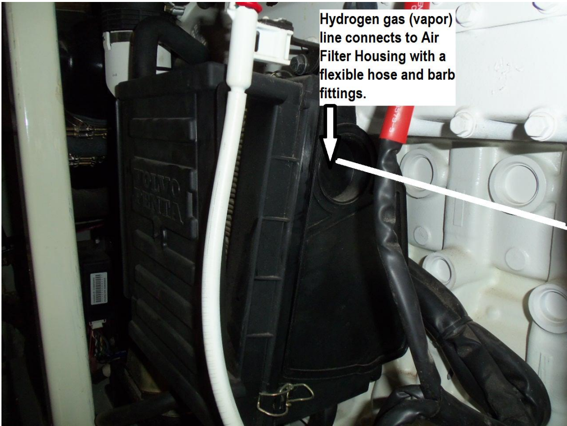
Hydrogen gas (vapor) line connects to Air Filter housing.
