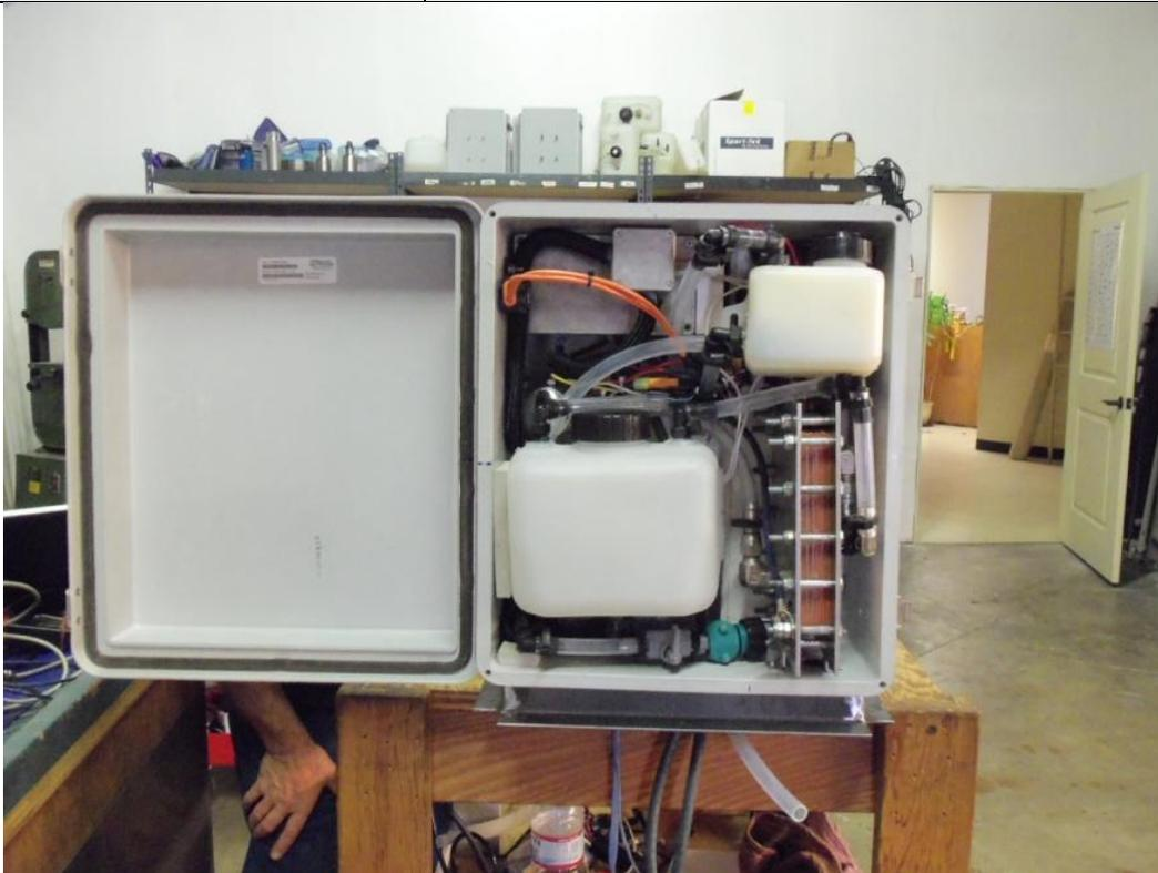
HPS recently completed an upgrade to its Series 300 that included adding heavy duty components that provide the ruggedness needed to withstand the pounding and vibrations associated with operating environment of larger vehicles.
